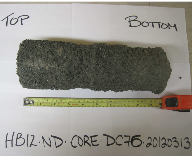
Photo 23: Drilled core 76
